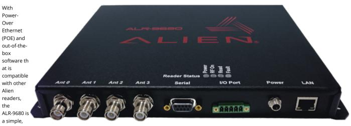
low profile solution that enables users to start reading tags and developing solutions immediately.
