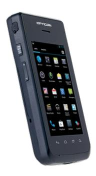
The H-27 delivers a powerful application performance thanks to the powerful 1.5 GHz processor, 8 GB flash memory and a range of communication possibilities. The powerful standard high capacity battery (2860 mAh) which is good for full-shift operation and the various communication options such as Bluetooth 4.0, WiFi, IEEE 802.11 a/b/g/n, 2.5G, 3.5G, NFC, GPS and GLONASS enable the mobile worker to provide a better and faster service on site.
