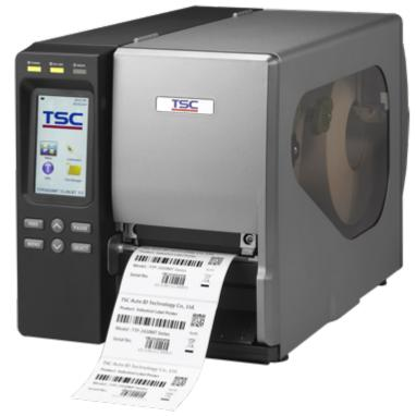
The TTP-2410M series is available in a 300-dpi model (TTP-346M), which operates at speeds up to 10 ips and can be ordered either from the factory or as a field upgrade. An upgrade kit, which includes a printhead and firmware, takes 30 minutes to install. Also available as a factory option is a 600 dpi model (TTP-644M), which operates at speeds up to 4 ips. Both the TTP-346M and TTP-644M offer 128 MB SDRAM, 128 MB Flash memory and an SD card slot for expanded memory.
